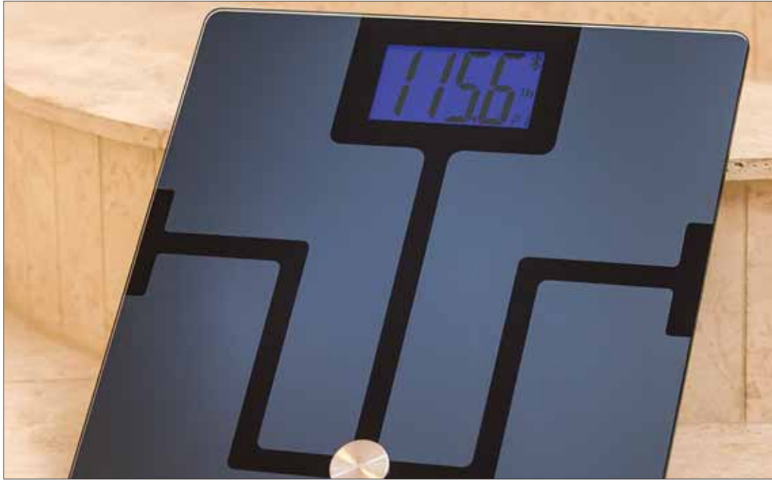
Bathroom scales like this Blueweigh Smart Body Composition Analyzer can also measure your basal metabolic rate (BMR) as well as body fat content, body muscle weight, water content, bone mass and more, but a lot of the calculations are really down to pure guesswork. Photo: Blueweigh
