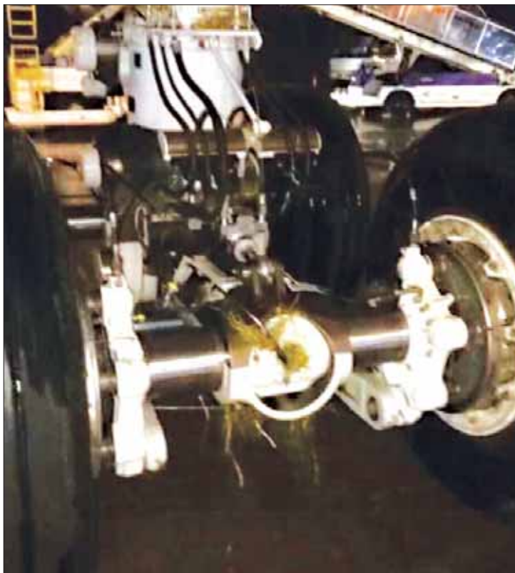
Grass and debris stuck to the damaged left-rear landing gear of flight TG 221, sustained after landing in Phuket. Photo: Ronnakorn Puttaraksa
